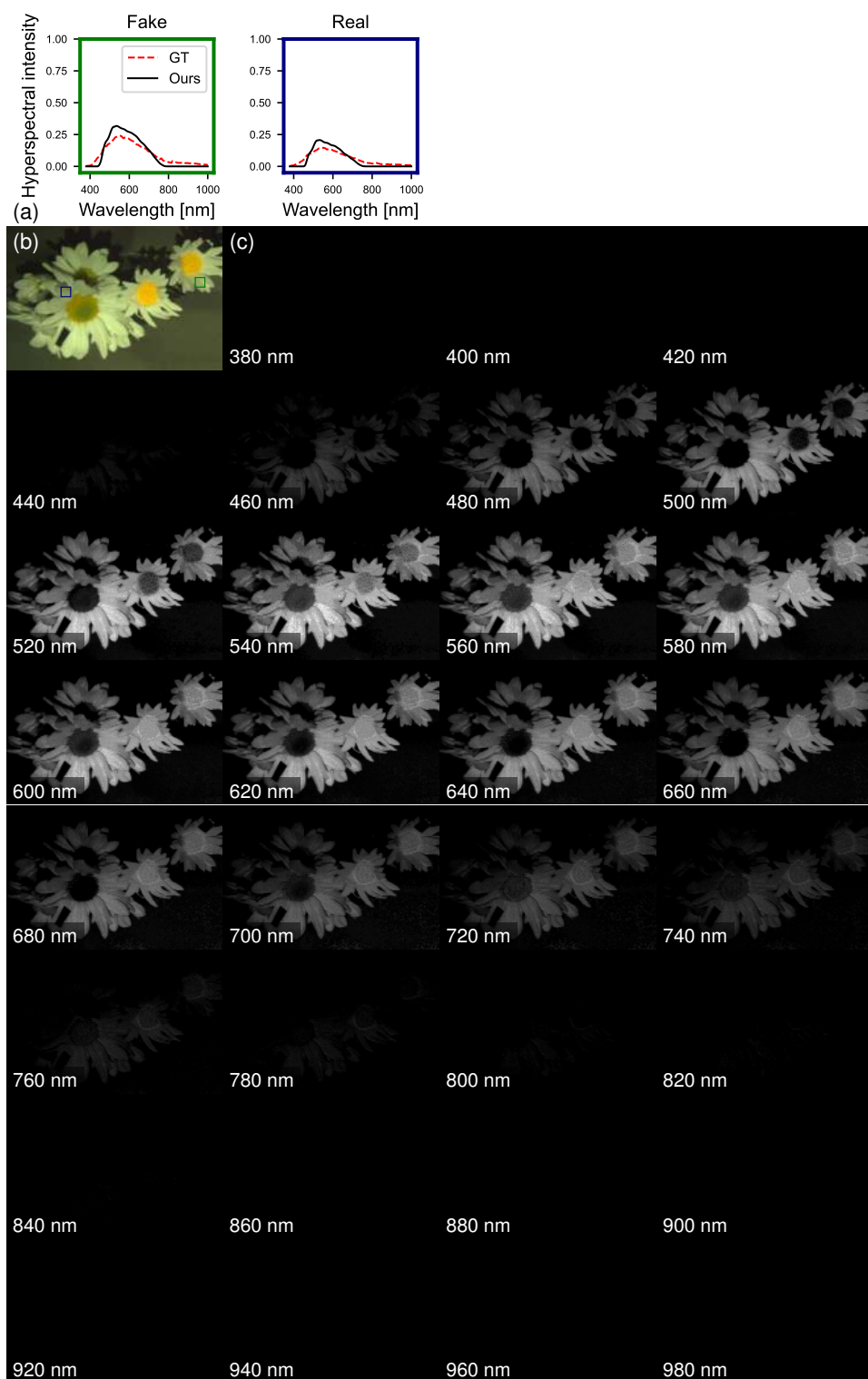
Figure 16. Evaluation of metamerism of real (left) and fake (right) white daisies. (a) Spectra of metamerism samples against ground truth measurements, highlighting the system’s ability to capture subtle spectral differences. (b) The reconstructed hyperspectral image in sRGB. (c) Estimated hyperspectral images.
