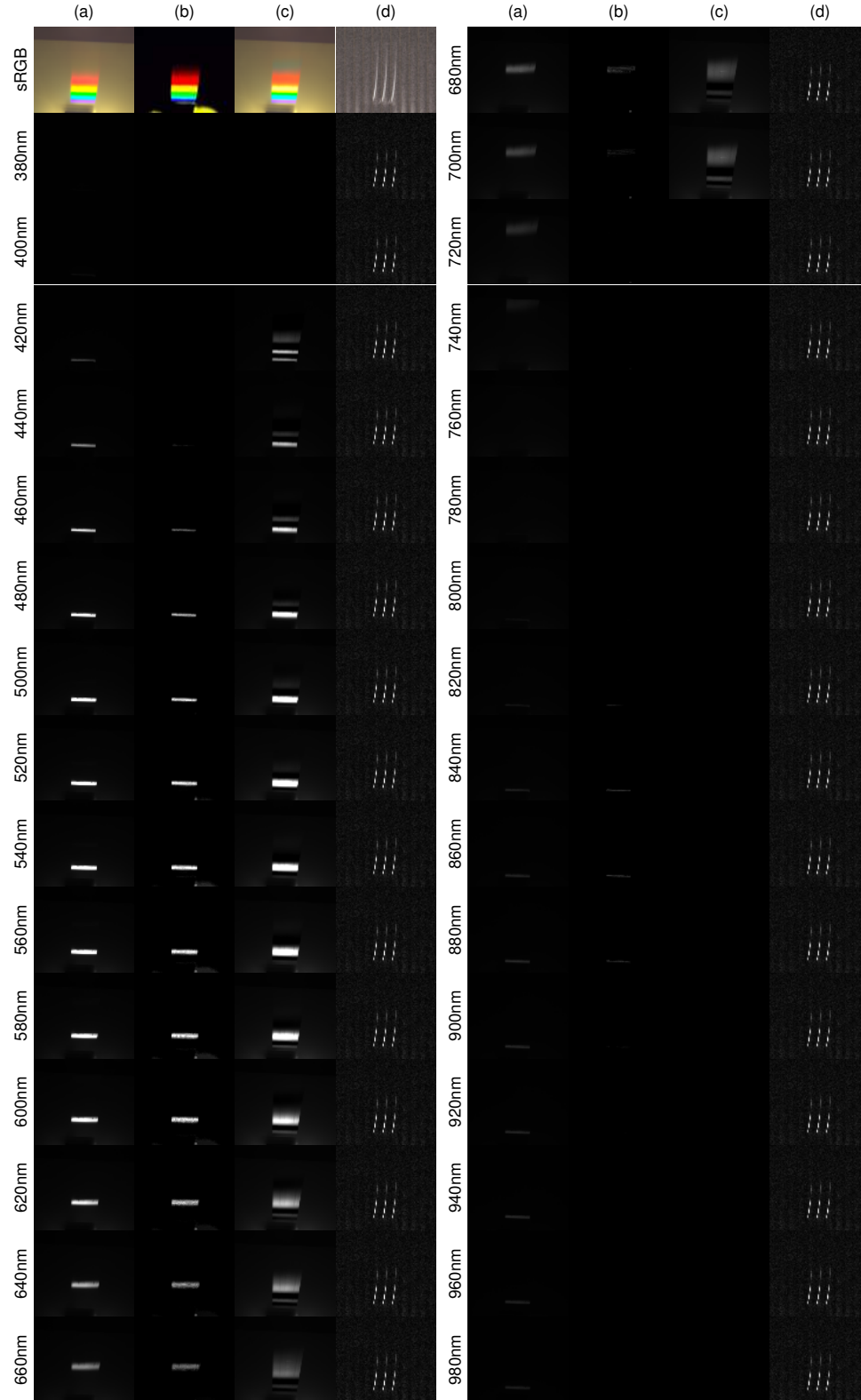
Figure 14. The full hyperspectral reconstruction results for examples in Fig. 5. Comparative analysis of spectral reconstruction on a high-frequency rainbow pattern. Compared methods include (a) ground truth, (b) ours, (c) basis-based method, and (d) bandwidth-matched frame-based method.
