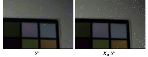
Figure 14. TFI-based SFR estimation and the corresponding result from adapted SpikeDiff pipeline. The white noisy points in recovered frames are caused by the out-of-distribution noise from TFI-based SFR estimation.
