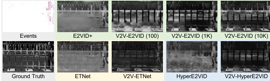
Figure 6: Qualitative comparison of reconstruction results on the EVAID Traffic sequence. Our method maintains information from camera motion occurred previously, even after it ceases.
