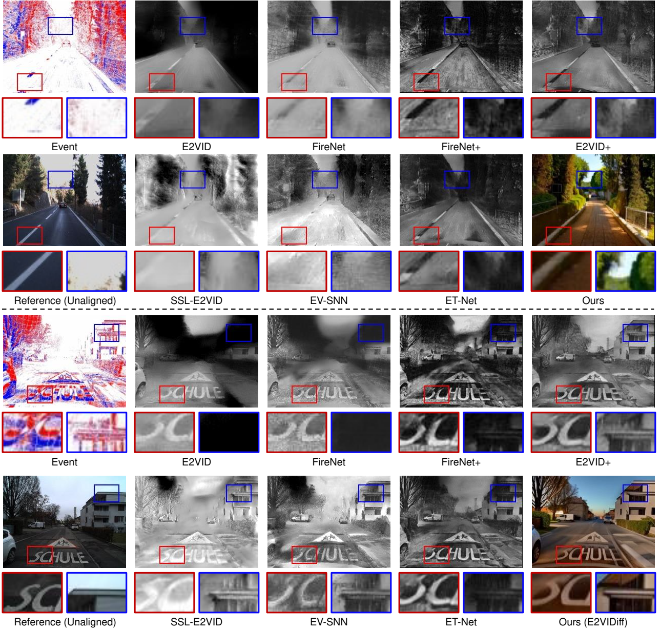
Fig. 5 Qualitative comparisons on real events captured by Prophesee Gen3 (Gehrig et al, 2021a) event cameras, accompanied by chromatic frames captured in stereo alongside the events, serving as unaligned references. Please refer to the caption of Fig. 4 for a complete list of the compared methods.
