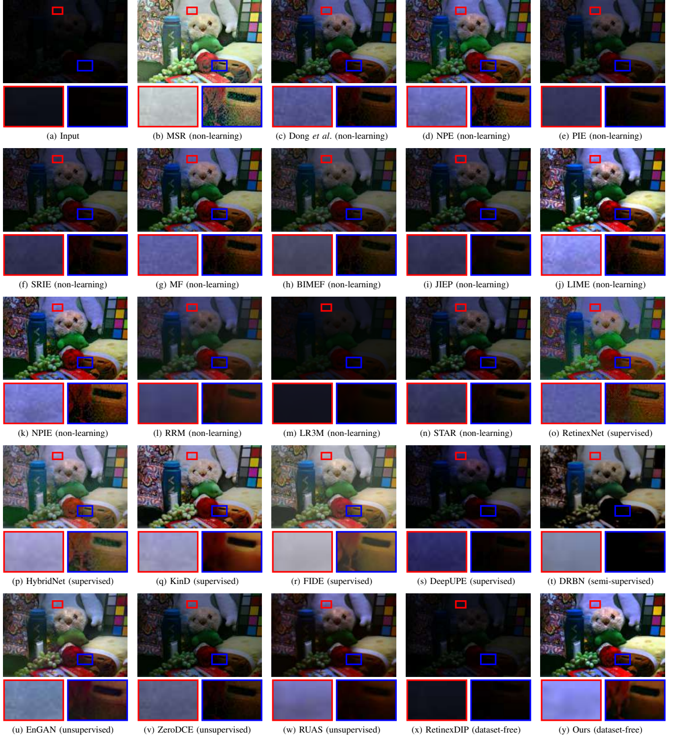
Fig. 6. Visual quality comparison of enhancement results. LIME and KinD can restore vivid color; however, it reveals significant noise (see e.g. , red boxes). KinD produces over-smoothed results in some regions (see e.g. , the ball of red wool in the middle), and the color of its result is less vivid in comparison to that of the proposed method and LIME. In contrast, the proposed method can enhance low-SNR regions while preserving color, even though it never sees any well/over-exposed images.
