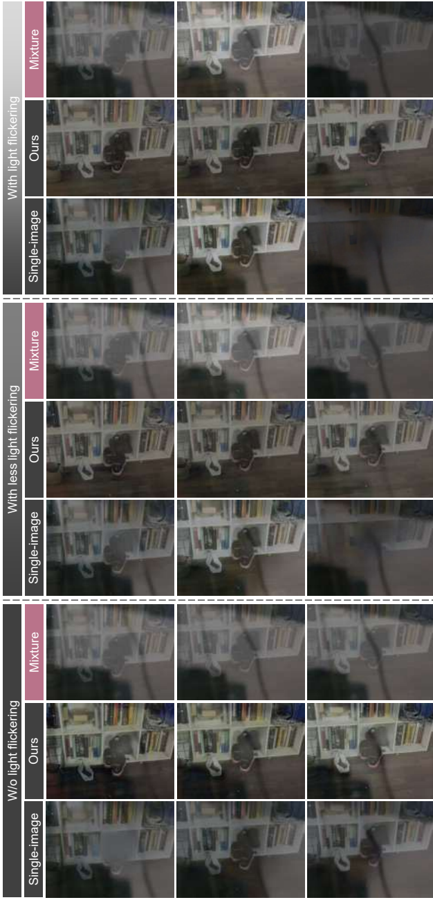
Fig. 18 Qualitative results of recovered transmission layers from mixture videos with different degrees of light flickering, compared with a single-image reflection removal method (Dong et al, 2021). Top part: The mixture video with light flickering and the reflection removal results. Middle part: The mixture video with less light flickering (the intensity of flickering is set at 40% of that in the top part) and results. Bottom part: The mixture video with no light flickering and results.
